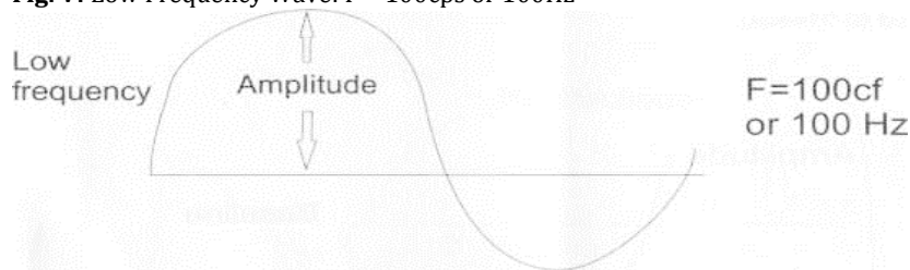
Fig. V: Low Frequency Wave: F = 100\text{cps} or 100\text{Hz}
